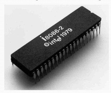
• The **greatest advantage** of the above processors are that it do not contain Floating point instructions. Here floating point refers to the radix point or decimal point. For example: 123.456 is a floating point representation. Processors such as 8085 and 8086 do not support such representations and instructions.
