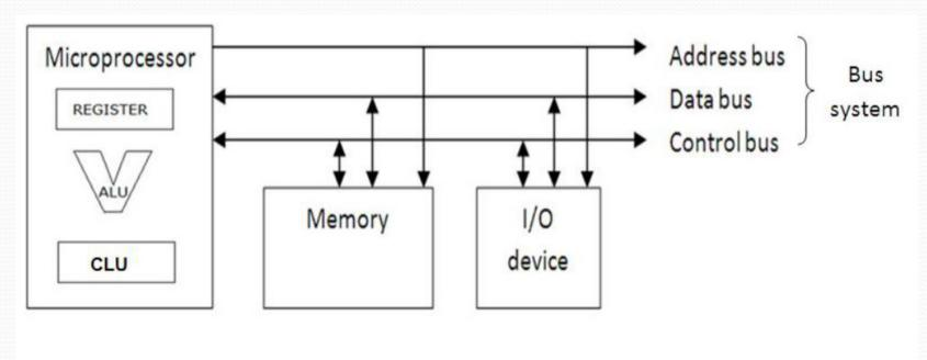
Figure 1.1 Microprocessor-based system
